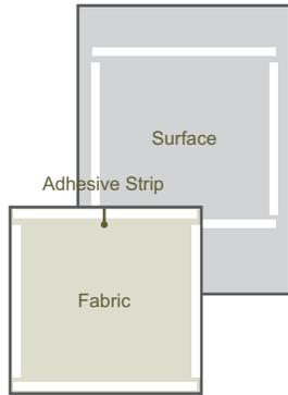
Sheer-Adhere Panels offer a simple way to attach a fabric to walls, glass, cement and stone.
